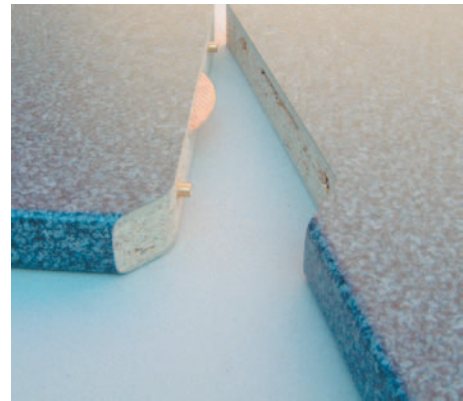
The use of our "fat" 12mm brass stud with an offset installation in this counter top made a knock-down installation possible where regular clamping could not have done the job.
